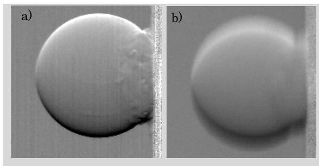
**Fig. 1.** X-ray differential phase images of a PMMA sphere ( $\phi = 3.2\text{mm}$ ) attached at the edge of a disk rotating at 5 rev/s. The sphere was moving at 1.4 m/s downward and captured: (a) stroboscopic with 8  $\mu$ s exposure time, and (b) non-stroboscopic with 0.3 ms exposure time.
