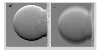
Fig. 1. X-ray differential phase images of a PMMA sphere ( $\phi$  = 3.2mm) attached at the edge of a disk rotating at 5 rev/s. The sphere was moving at 1.4 m/s downward and captured: (a) stroboscopic with 8 µs exposure time, and (b) non-stroboscopic with 0.3 ms exposure time.
