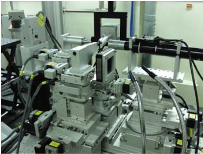
Fig. 1. The fresnel zone plates hard x-ray nano-focusing system.
