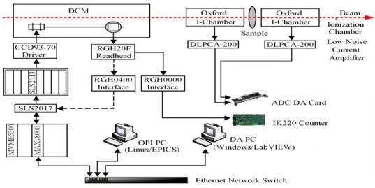
Fig.1 Schematic of QXAFS system at BL14W1
